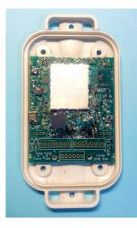
External sensor connection is by means of a compact multi-pin header which provides all the signals needed for sensors, actuators or switches. The device itself is low powered and can be used on external power, standard batteries or rechargeable Lithium battery using the on board USB charger. It is available in robust enclosures either outdoor or indoor types.
